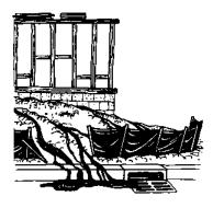
A poorly installed silt fence will not prevent soil erosion. Fabric must be buried in a trench and sections must overlap (see diagram on back of this fact sheet).
